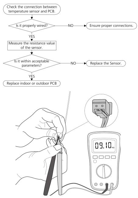
Note: For certain models, outdoor PCB could not be removed separately. In this case, the outdoor electric control box should be replaced as a whole. This picture and the value are only for reference, actual appearance and value may vary
